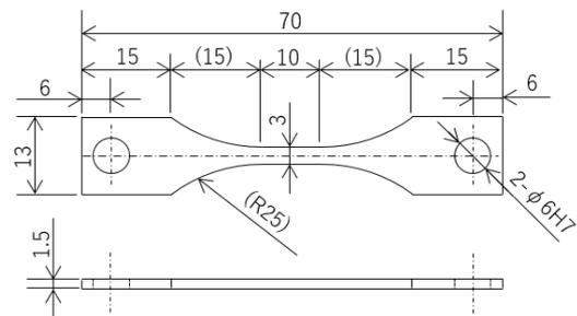
Fig. 1 Specimen Shape and Size (Dimensions in mm)
