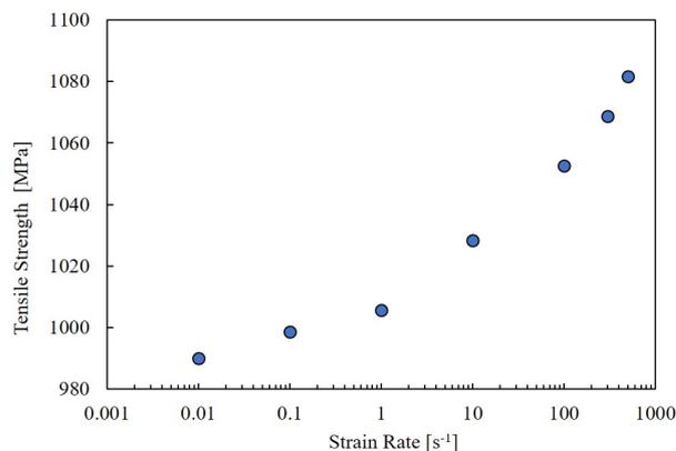
Fig. 5 Tensile Strength-Strain Rate Relationship (Mean Value)
