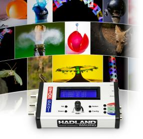
**Hadland modified StopShot** with 3 BNC connectors for interfacing with high-speed & ultra high-speed cameras.
