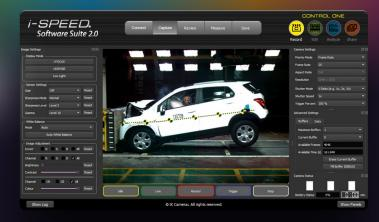
**Video Trigger** – The latest feature of the i-SPEED Software Suite 2.0 lets you define trigger levels in manual mode or choose auto mode and have the software calibrate trigger levels for you. A real-time track mode has been added for triggering the camera in a dynamically changing environment such as cloud cover.
