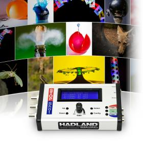
**Hadland modified StopShot** with 3 BNC connectors for interfacing with high-speed & ultra high-speed cameras.
