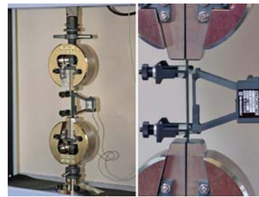
Fig. 2 Experimental set up for tensile tests
