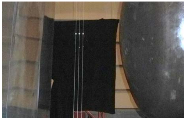
Fig.3. Three metal balls of 3/4" diameter separated by 3/4" spaces and suspended in a uniform E-field of 1 \text{ MV m}^{-1} between the negative high-voltage (on the right) and the ground (on the left) electrodes.
