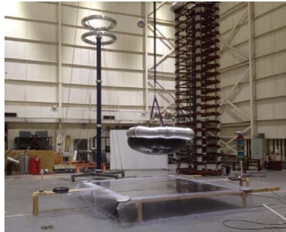
Fig.7. The setup for the second phase of the experiment at the high-voltage facility at Mississippi State University. The ambient E-field between electrodes in the 0.9 m wide gap is vertical; the particles were suspended on horizontal dielectric threads.
